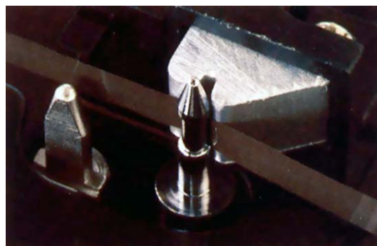
Fig. 17 – Back tension pin, combined with the tape guide (Hitachi D-3500).
