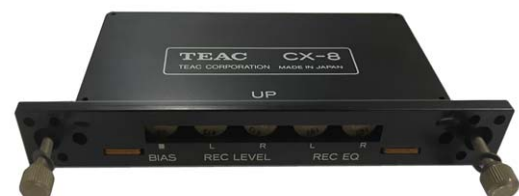
Fig. 28 – Replaceable calibration card TEAC CX-8.
