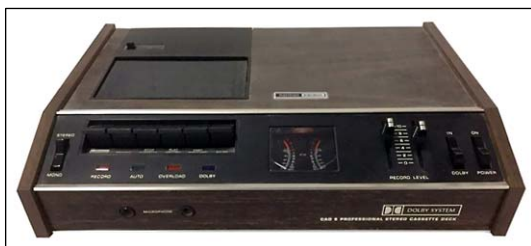
Fig. 9 – Harman/Kardon CAD5. The first cassette deck with Dolby B.
